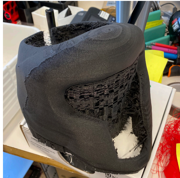
34. Fully TPU Printed Model with Supports and Faulty Seam Line
