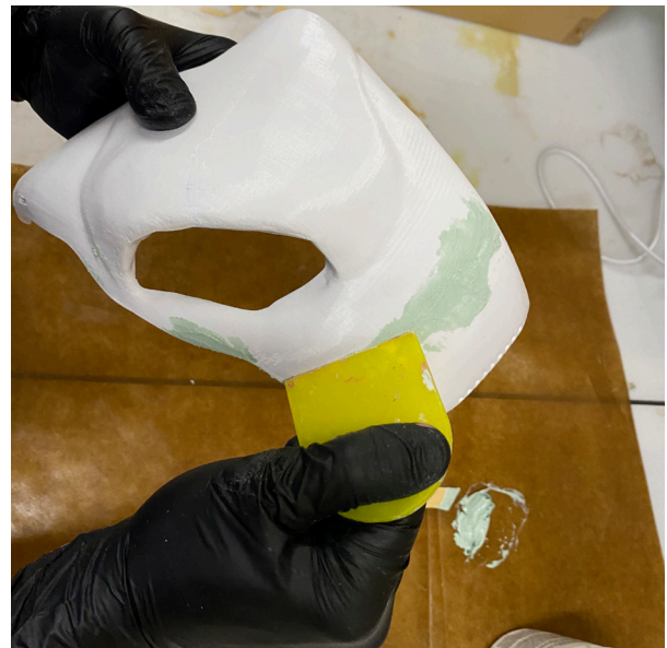
31. Applying and Cleaning Bondo from the Headgear
