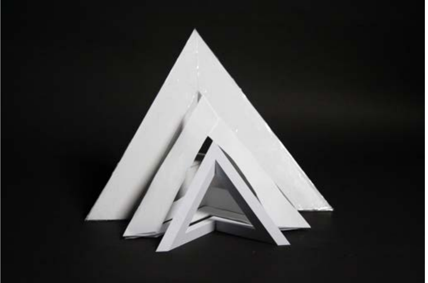
Trio of models. Front to back 3D print(PLA plastic), paper model, foam core positive. 3D print sitting in foam core positive.
