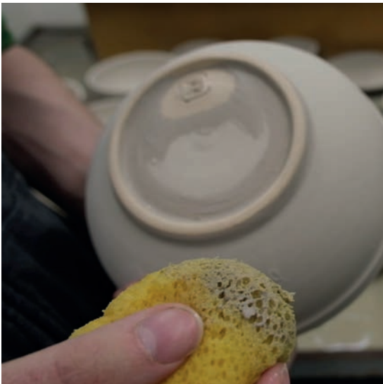
Cleaning off the glaze from the feet to prevent sticking to the kiln shelf (Fig 93.)
