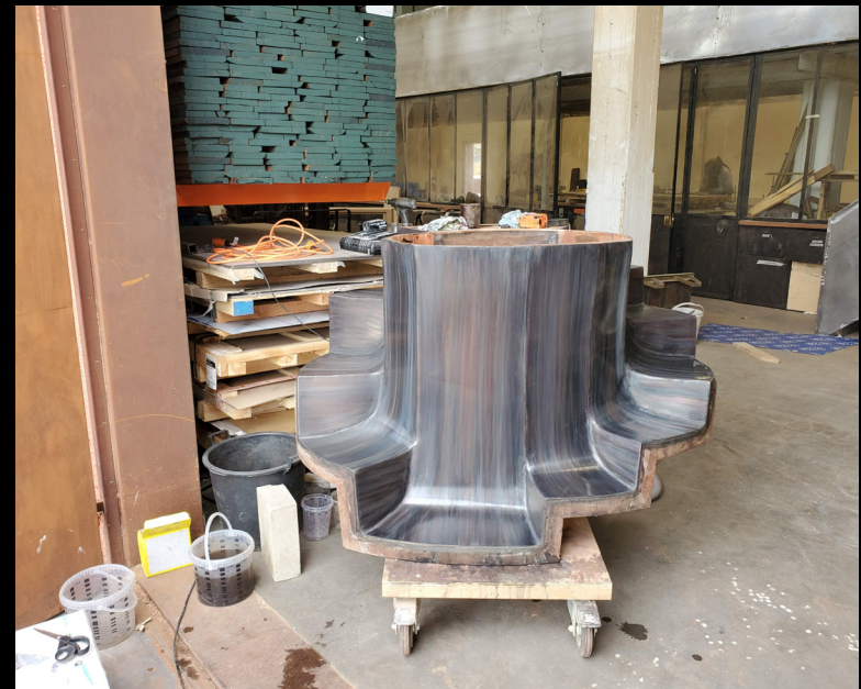
fig. 11 Copper and Walnut Staircase after patinating
