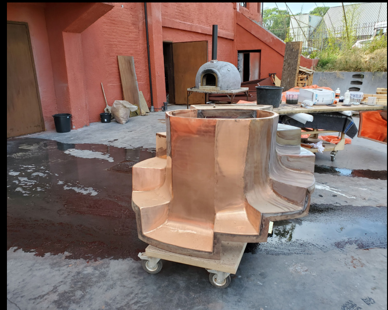
fig. 10 Copper and Walnut Staircase before patinating
