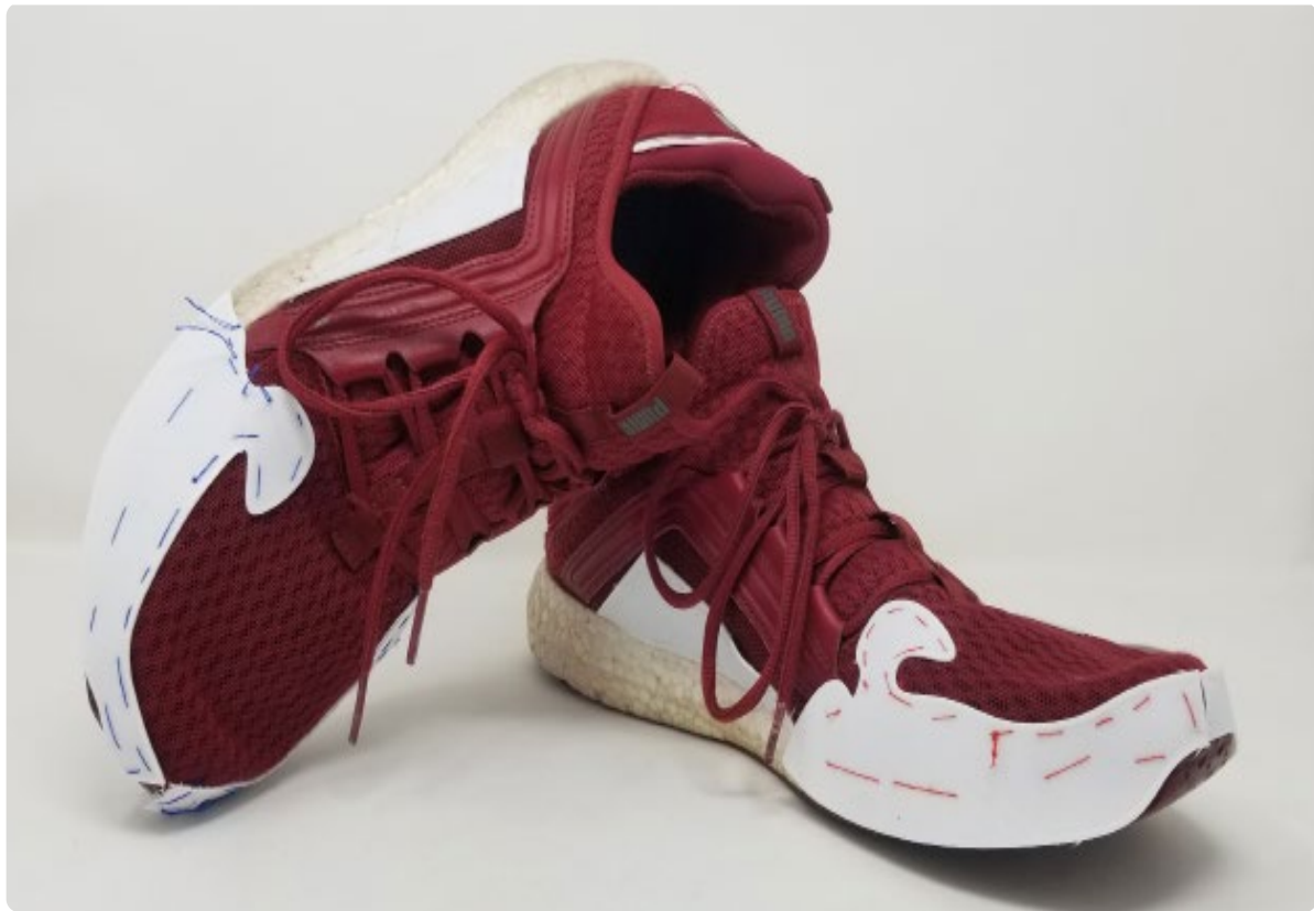
Figure 33: Shoes stitched with TPU reinforcements [Photo : Devya Patel]
