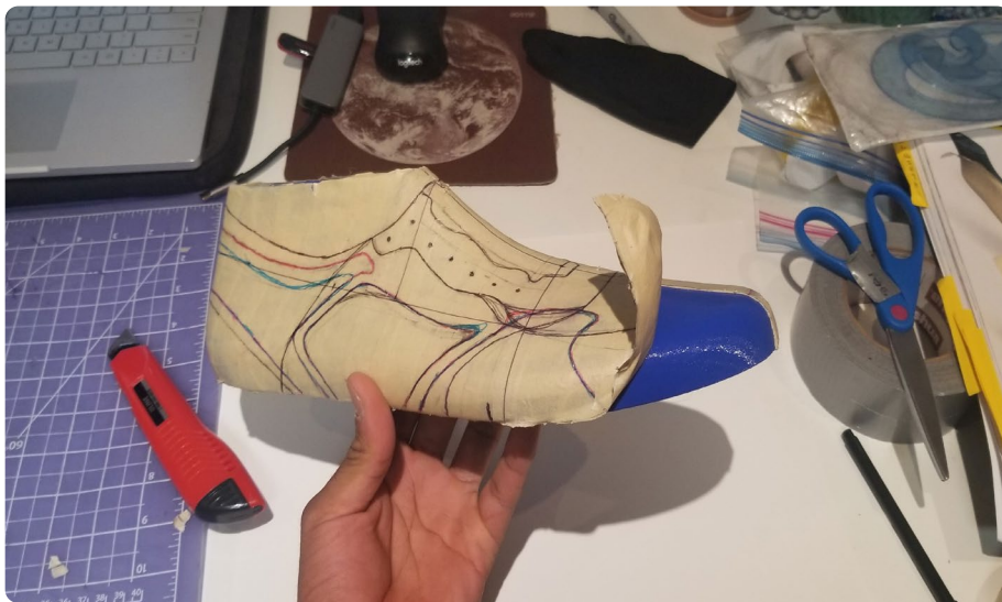
Figure 43: Pattern Drawing on the Last [Photo: Devya Patel]
