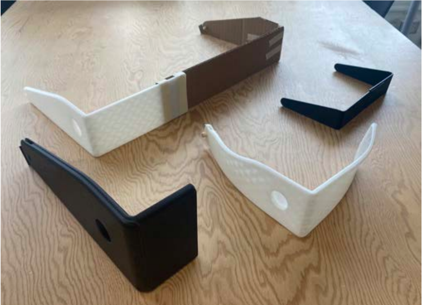
Testing a variety of angles and heights for the stove guard through PLA printing.
