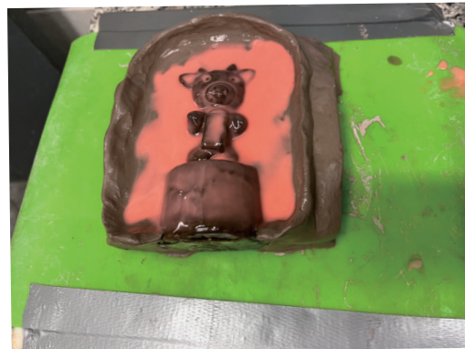
Spray mold release agent and put rubber on the model a layer and a layer, and dry out
