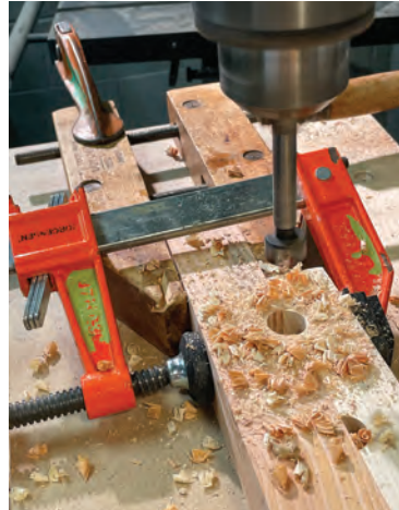
fig. 57 Drilling holes for the back rest rails
