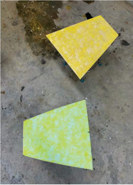
fig. 67 Spray adhesive on the foam and plywood
