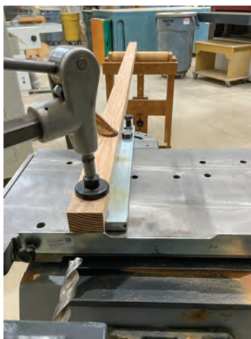
fig. 49 Mast set up on the slot mortiser
