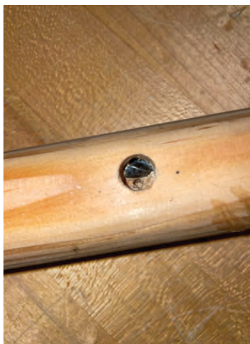
fig. 50 A sunken treasure, a drill bit dislodged and embedded in the mast
