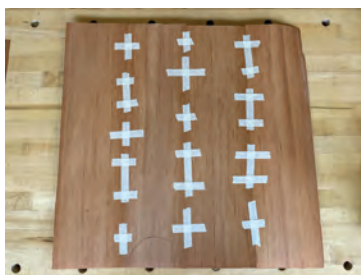
fig. 61 Jointed veneer ready to be glued
