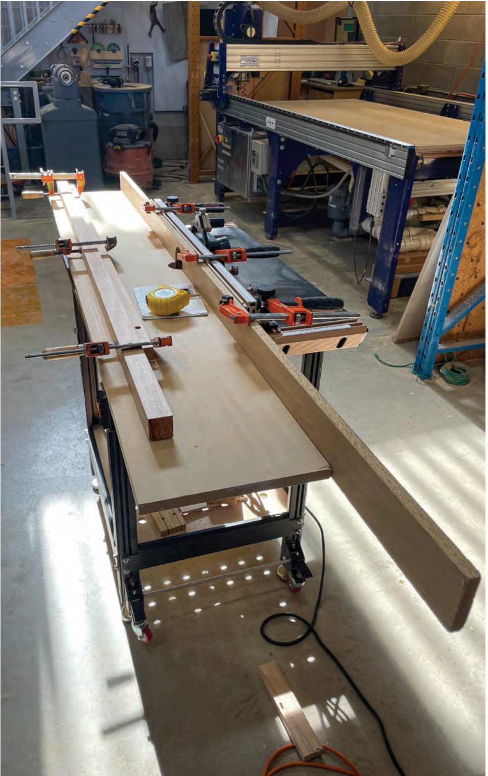
fig. 51 Setting up the router table for round overs
