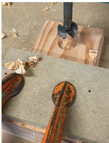
fig. 60 Drilling holes in the anchor
