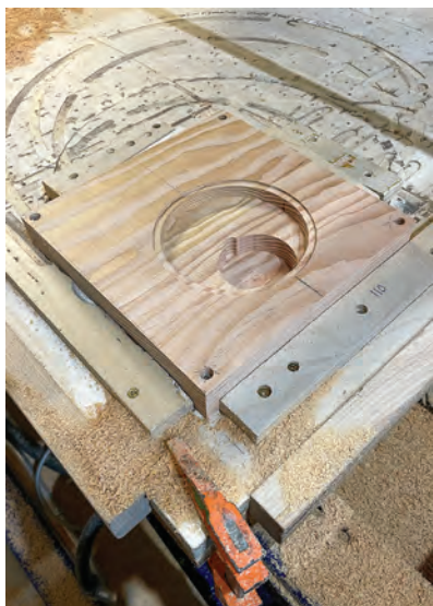
fig. 53 Bottom of the light base on the CNC
