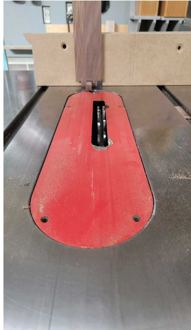
Figure 64: Finger joint set up
