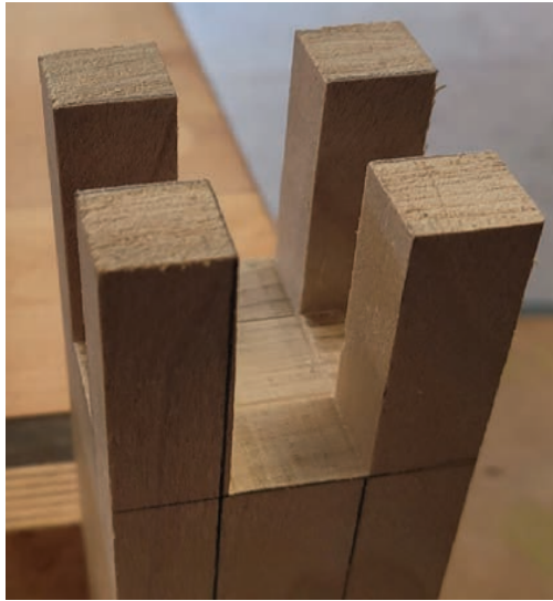
Figure 18: Castle joint in progress
