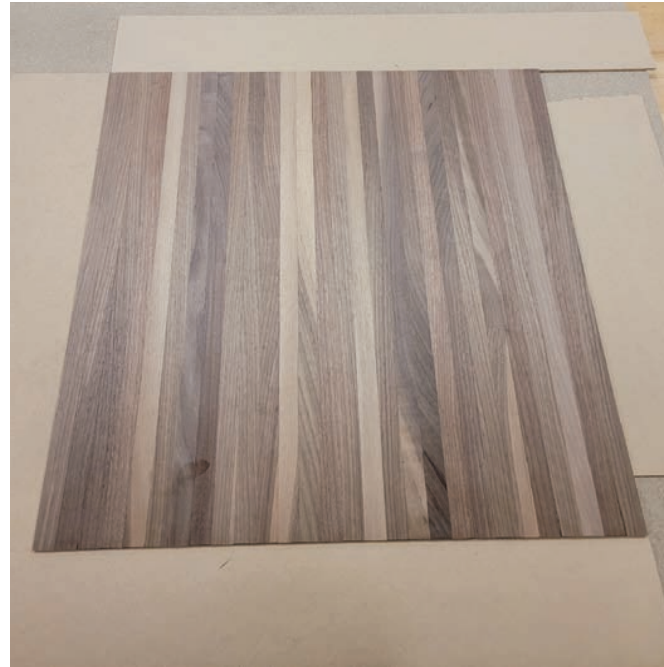
Figure 65: Tambours in jig
