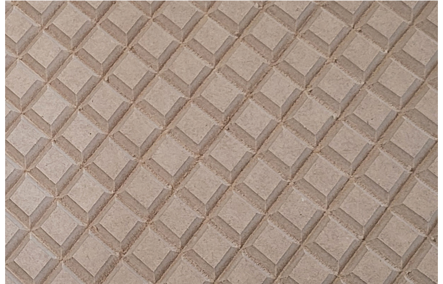
Figure 33: Deeper thistle texture CNC tests
