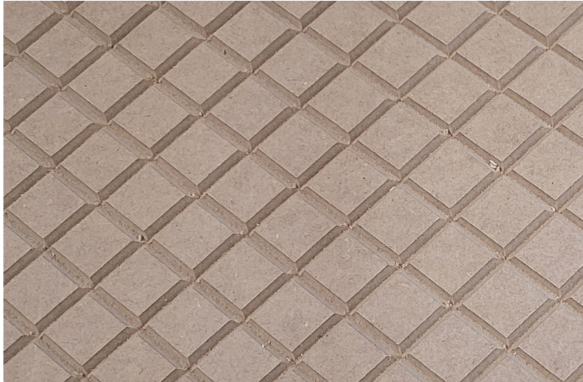
Figure 32: Thistle texture CNC tests
