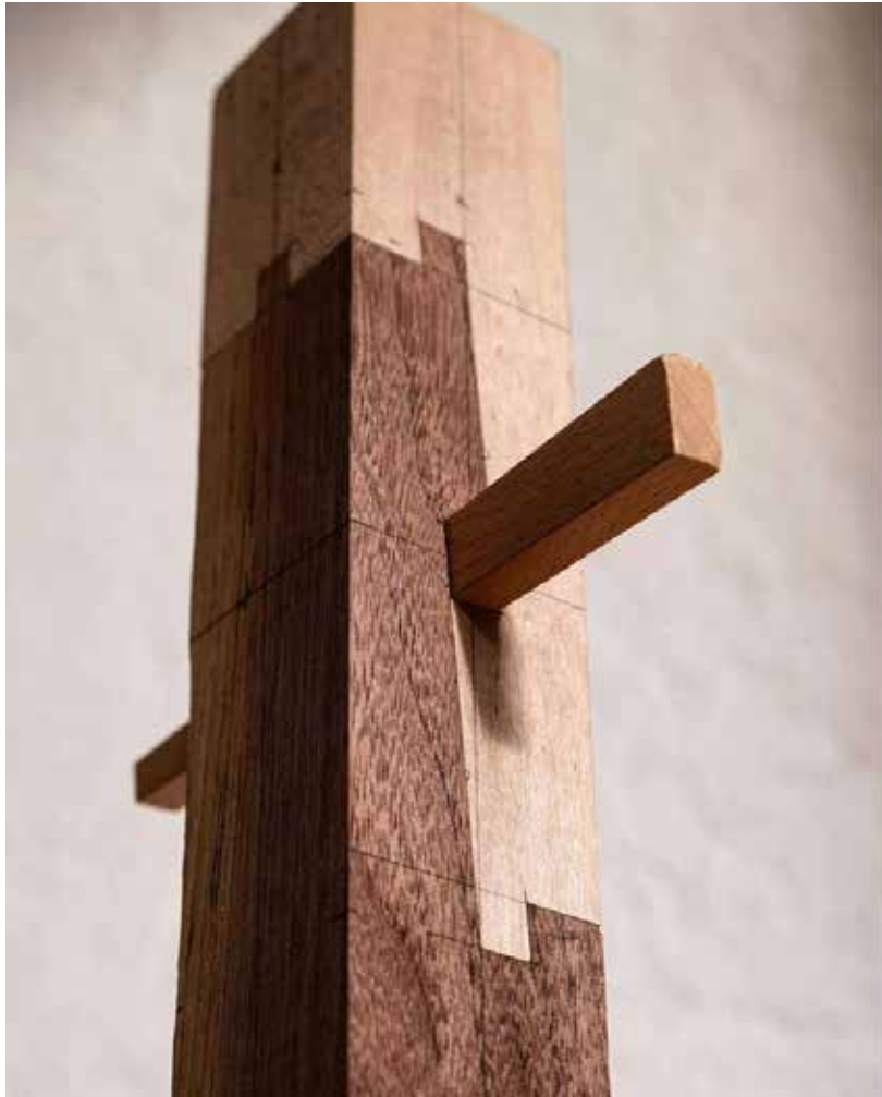
Figure 13 - Kanawa Tsugi joint by Dylan Iwakuni
