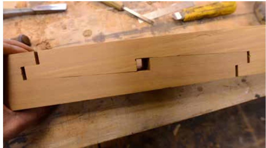
Figure 14 - Kanawa Tsugi joint
