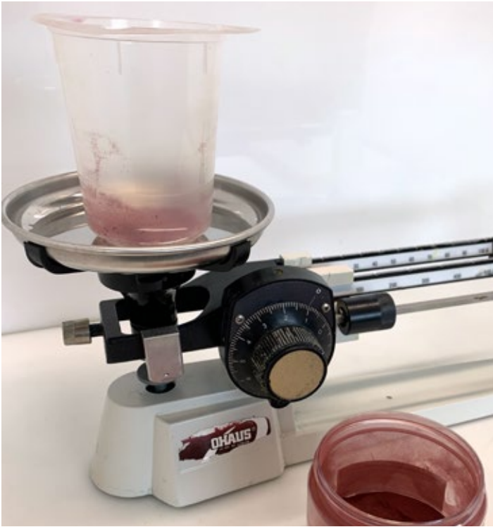
Fig. 80 : Cochineal extract is weighted out at 2% weight of fibre. Marigold is weighed out at 5%.
