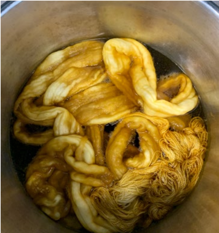
Fig. 67 : Wool roving and silk yarn are immersion dyed for 30 minutes at 60°C.
