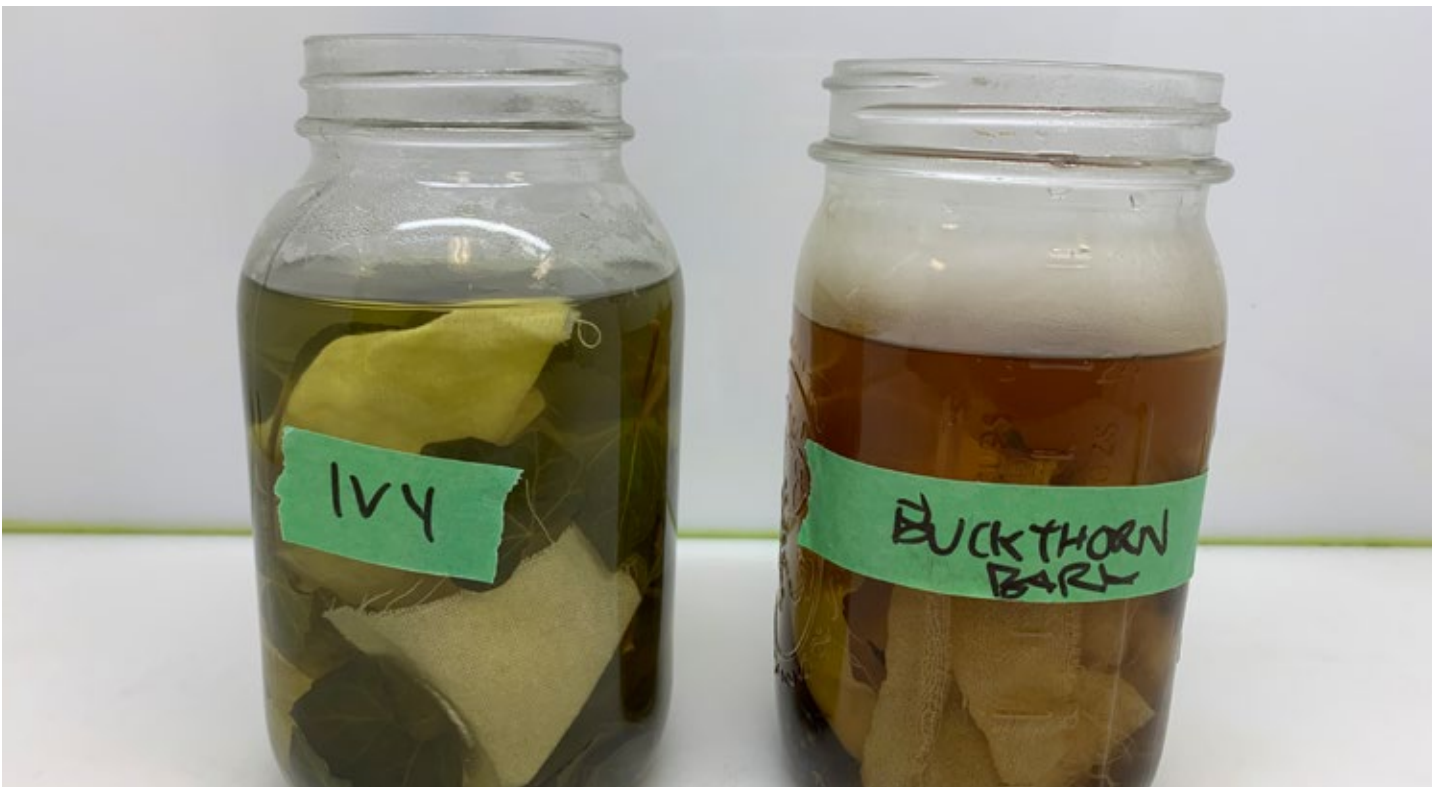
Fig. 19 : English ivy and buckthorn bark dye baths with cotton, silk and wool swatches.
