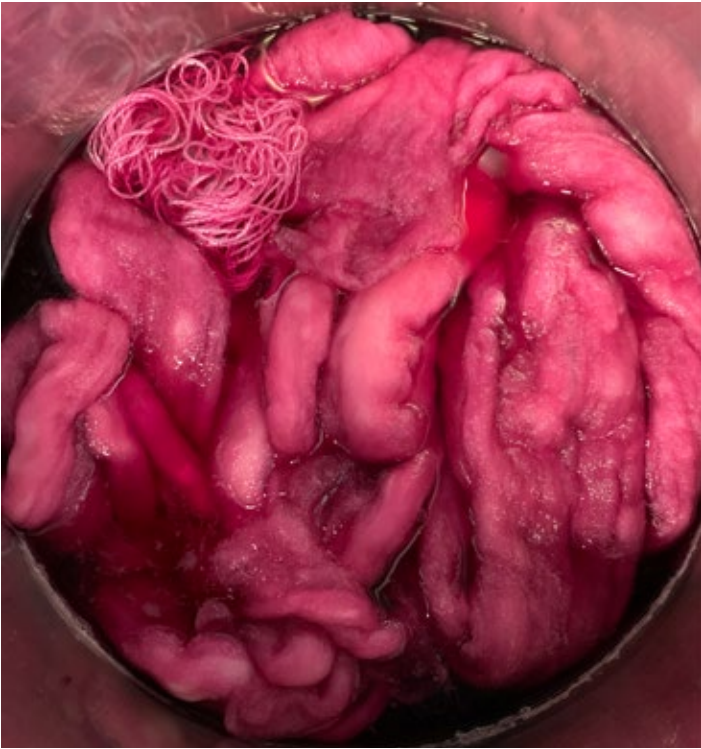
Fig. 71 : Wool roving and silk yarn are immersion dyed for 30 minutes at 60°C.
