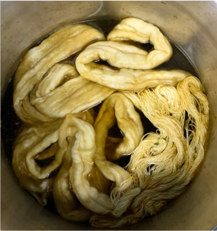
Fig. 86 : Roving and silk yarn are immersion dyed for 10 minutes at 60°C in marigold bath.
