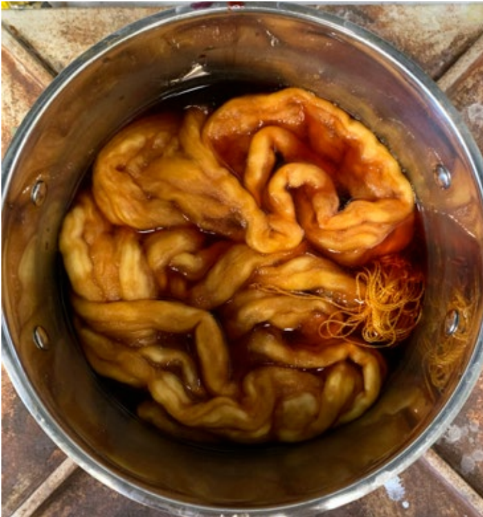
Fig. 77 : Cochineal extract is dissolved in hot water and added to marigold bath. The fibres are immersion dyed for 30 minutes at 60°C.
