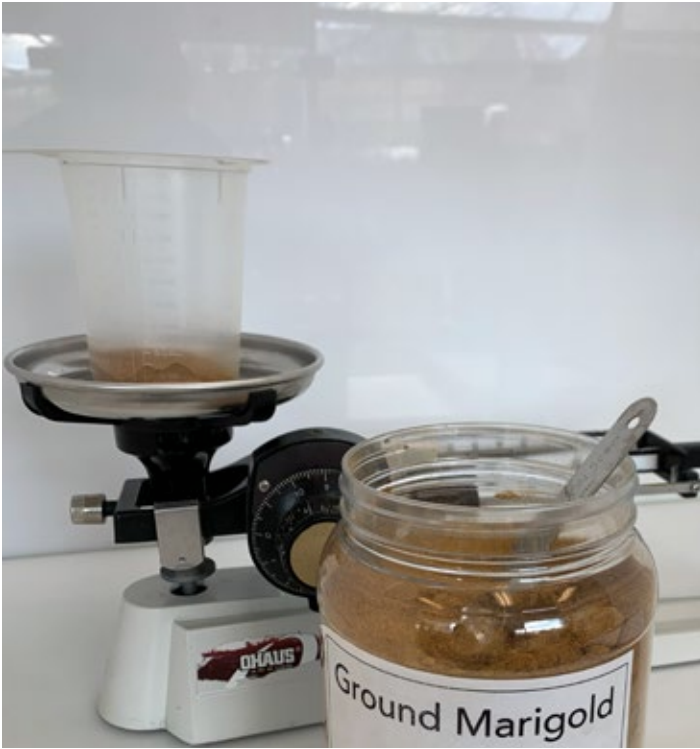
Fig. 75 : Marigold grounds are weighed out at 10% weight of fibre. Cochineal is weighed out at 0.25%.
