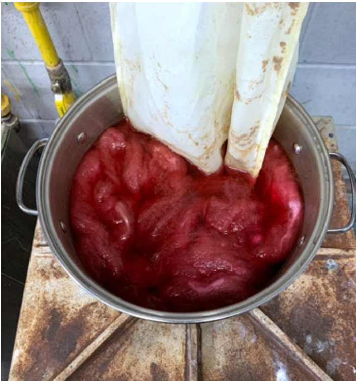
Fig. 82 : Fibres are immersed while extracting the marigold grounds in a mesh bag to ensure a very light deposit of yellow dye.
