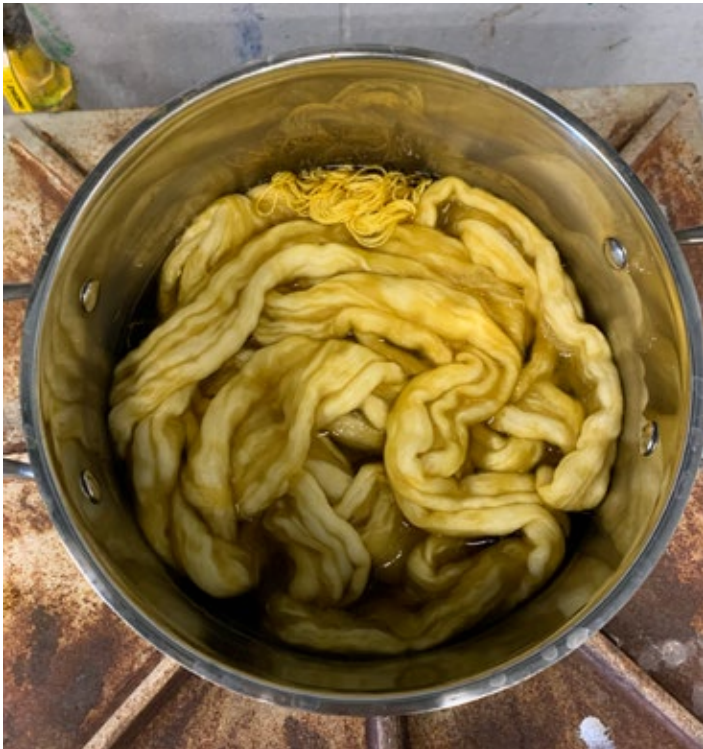
Fig. 76 : Marigold is extracted in a mesh bag for 30 minutes. The bag is removed and fibres are added.
