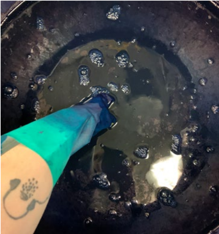
Fig. 87 : Fibres are dipped in an indigo workhorse vat twice for 2 seconds, then thoroughly rinsed.
