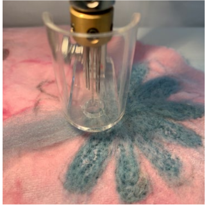
Fig. 17 : Wool roving is felted into the surface of cotton velveteen using an embellishing machine.
