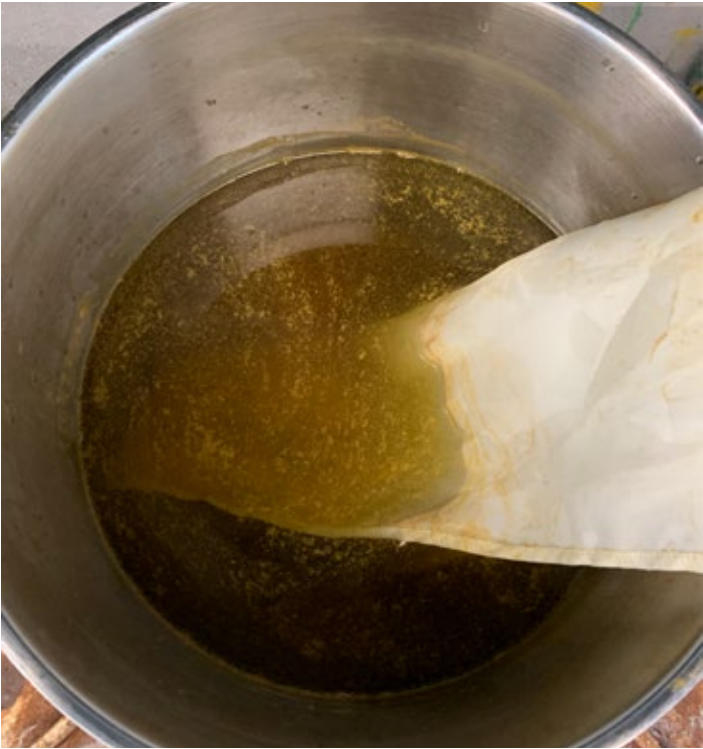
Fig. 66 : Grounds are placed in a mesh bag and dye is extracted at 60°C for 25 minutes.
