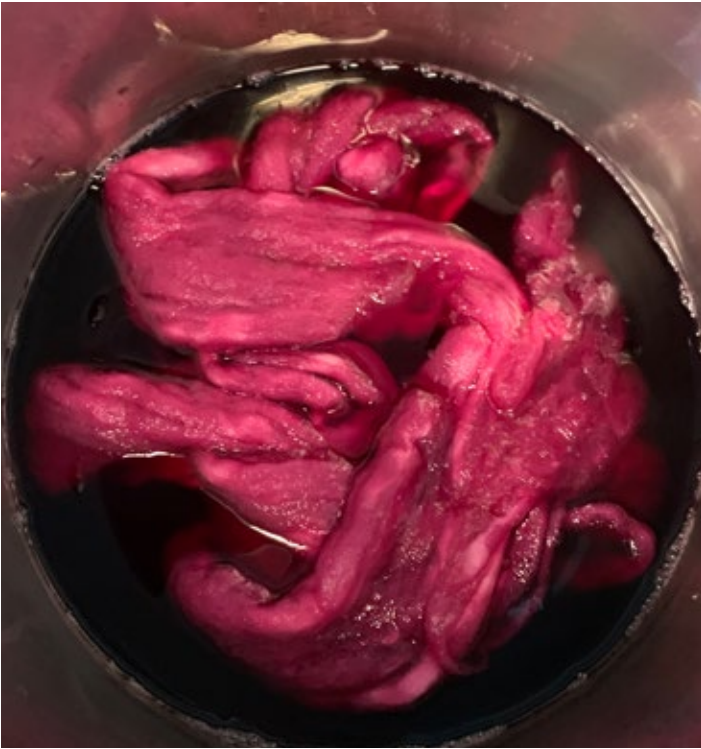
Fig. 81 : Roving and silk yarn are immersion dyed for 30 minutes at 60°C in cochineal bath, then removed
