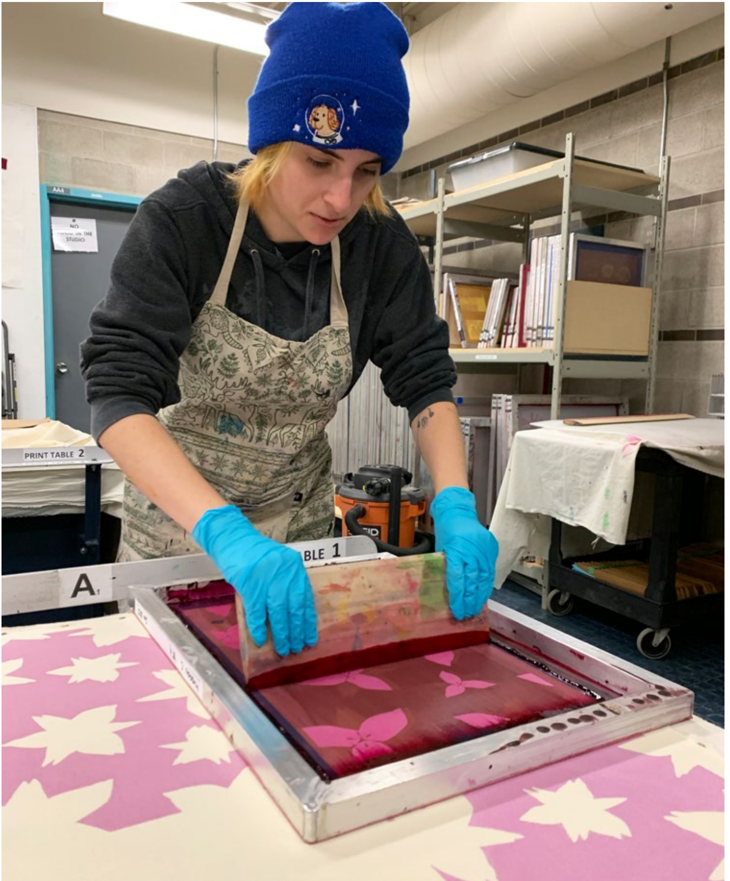
Fig. 58 : Printing the Red Trillium print's background screen with cochineal natural dye paste.
