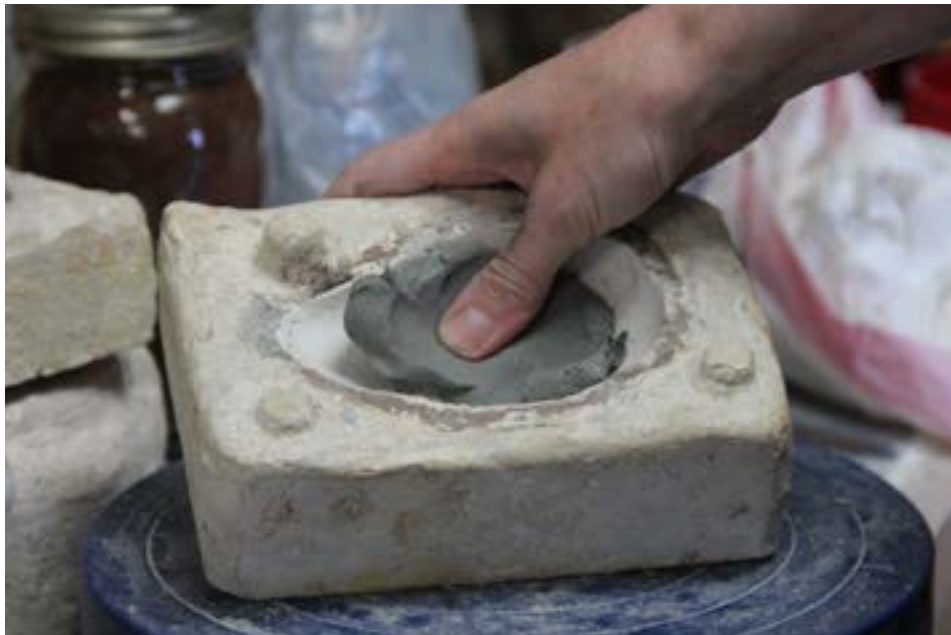
2.5 Rachel Dorn. Press Moulding with plaster mould
