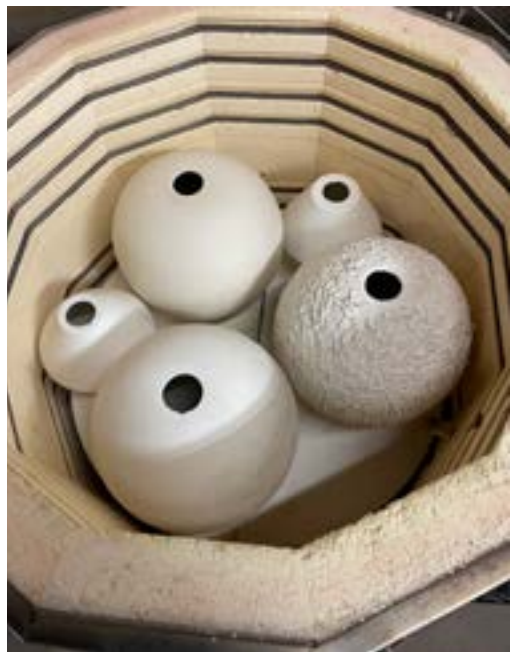
Ceramic shades were placed into a kiln and bisqued to cone 06.
