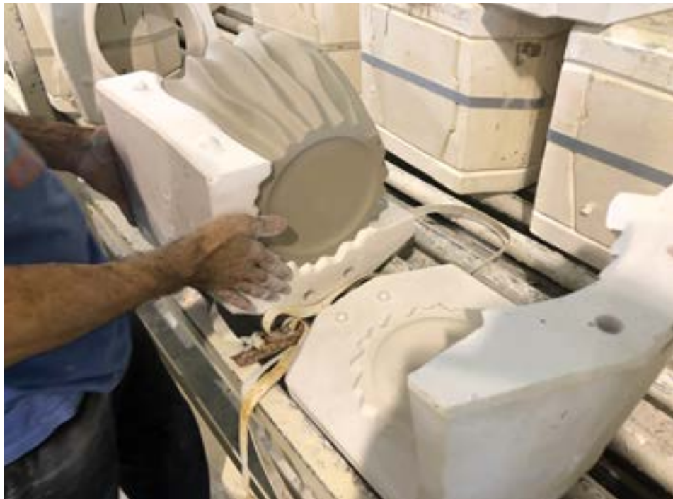
2.3 Removing greenware from plaster mould - Sporvil Ceramics
