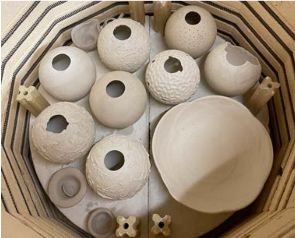
Ceramic shades were placed into a kiln and bisqued to cone 06.
