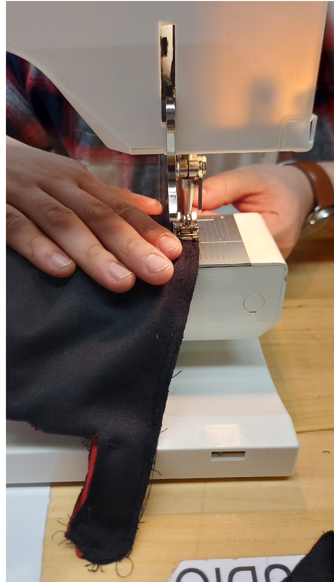
Sewing the final seam to complete glove
