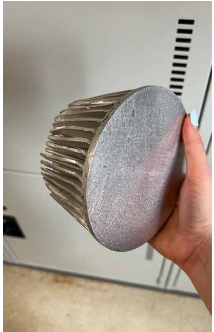
Cutting both the heatsink and cooper plate to fit my working model
