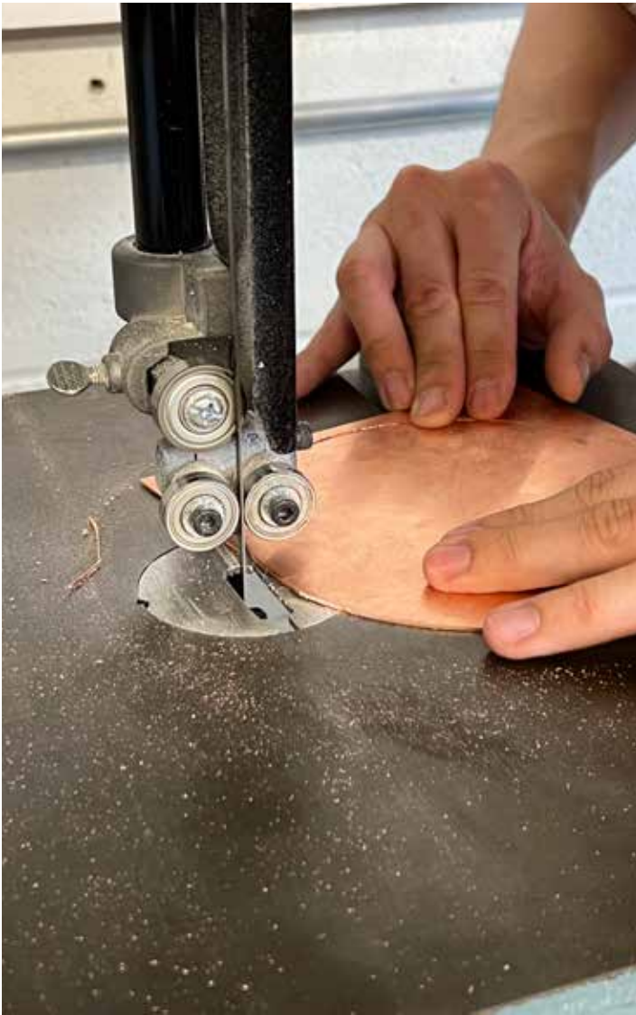
Cutting both the heatsink and cooper plate to fit my working model
