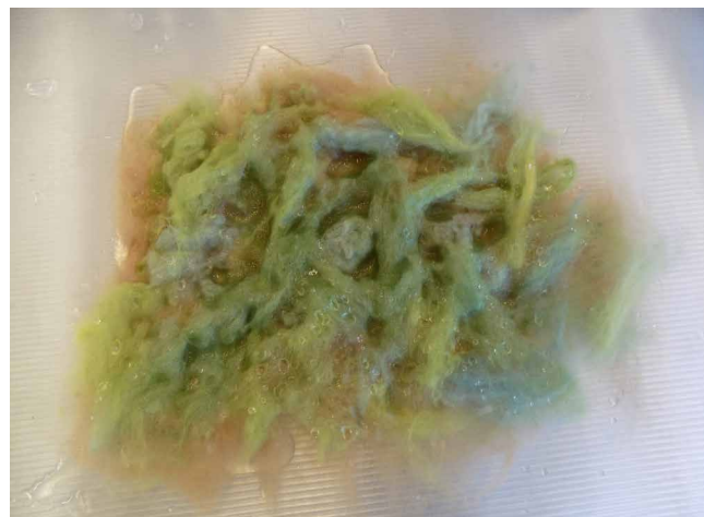
Fig. 26 - Fibers wetted out using hot water.
