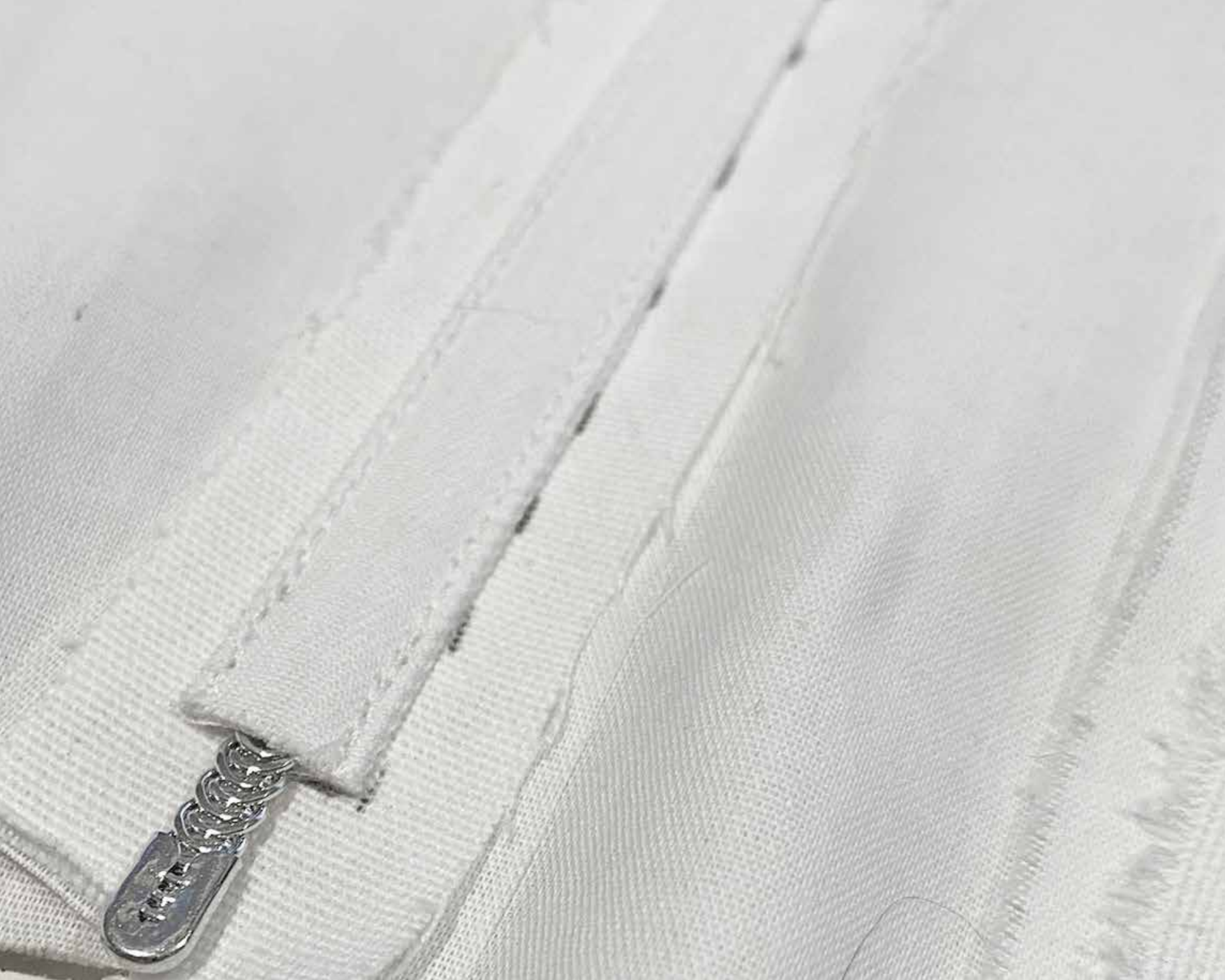
Figure 54: The boning and casing lined up along the dashed lines on the inside of the corset lining
