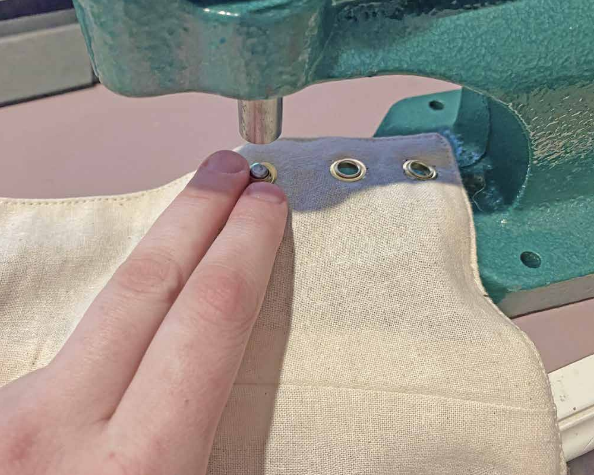
Figure 40: Grommets being inserted into the corset to allow lacing to pass through
