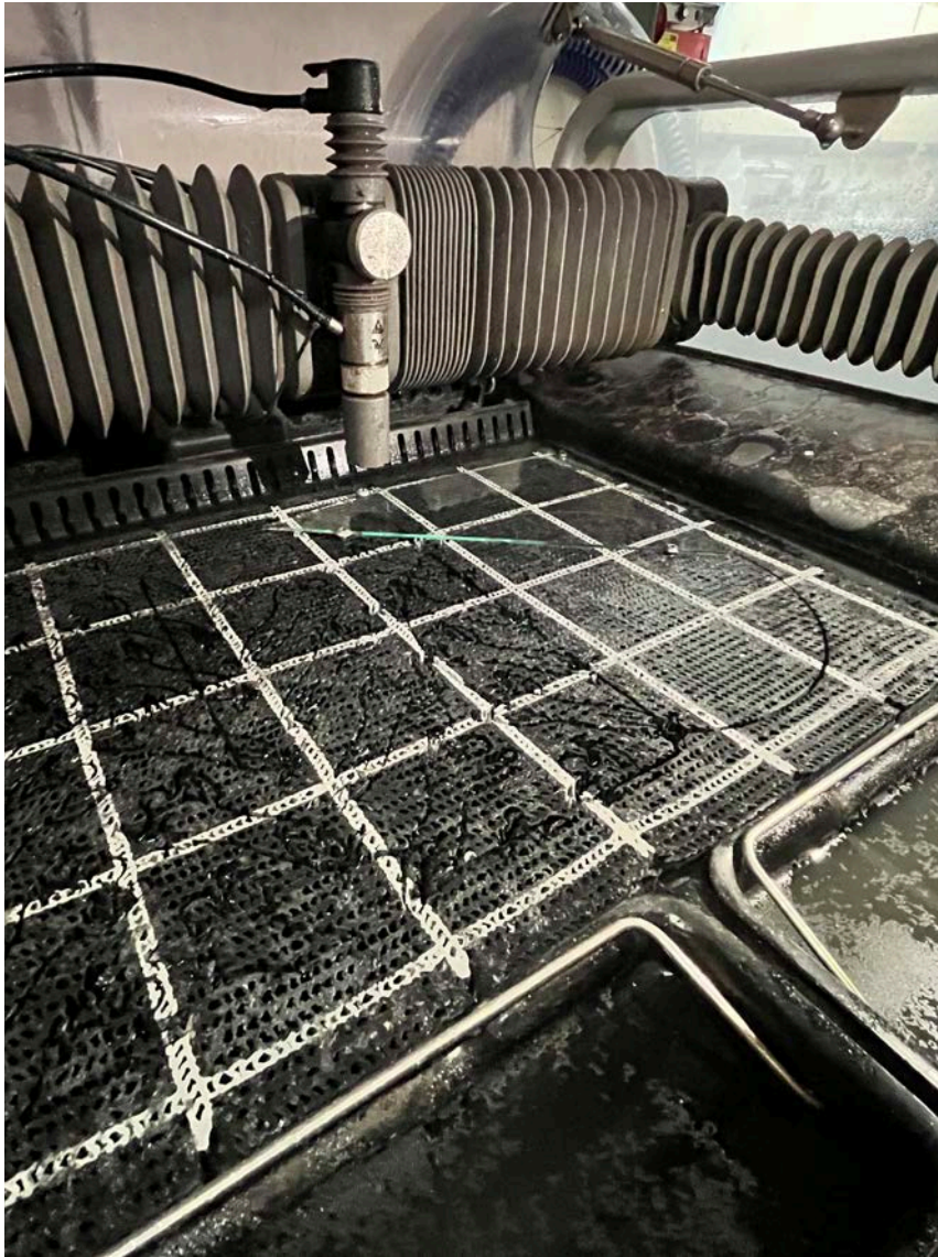
Lenses were cut from glass sheets with the Waterjet to be used for the face of the wrist monitor
