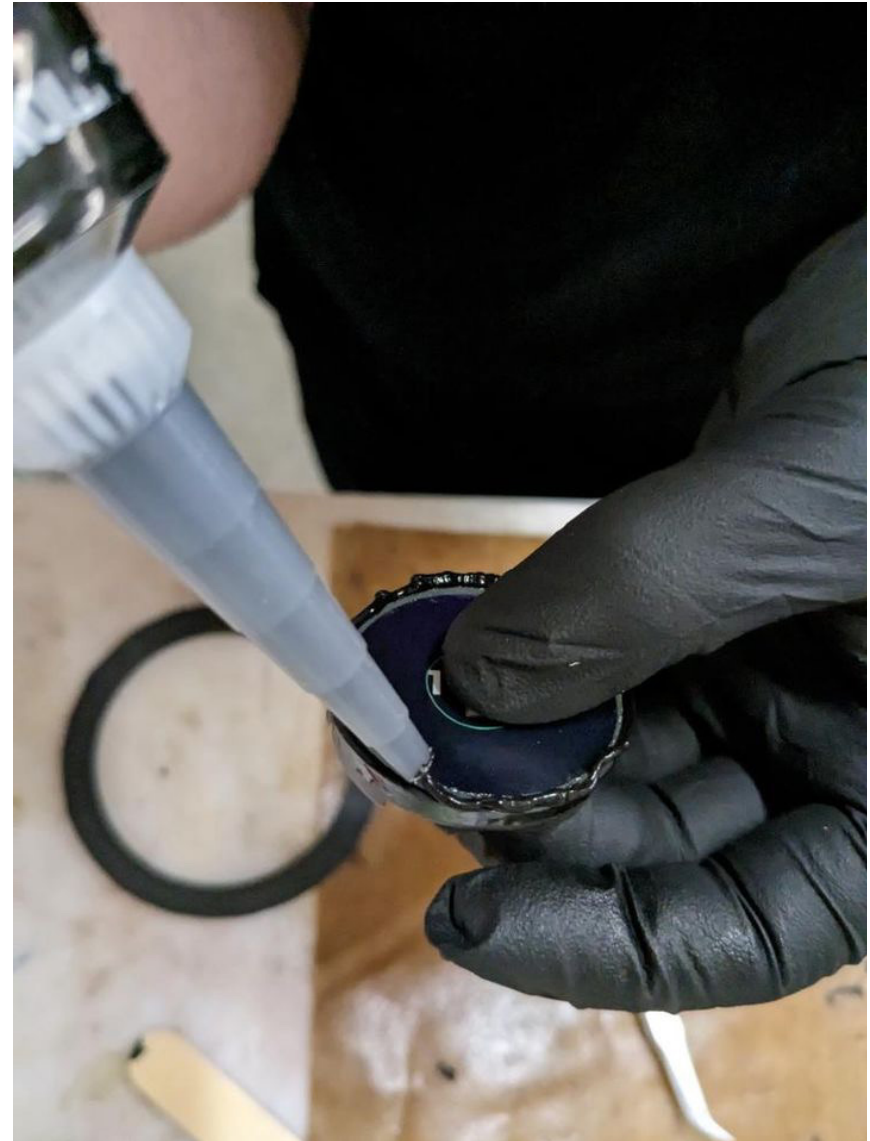
To secure the glass in the monitor housing, a bead of black silicone was used around the edge and later cleaned up with rubbing alcohol
