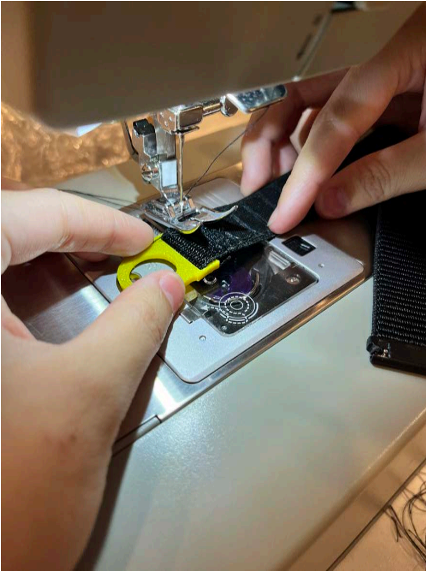
The pull tab of the wrist monitor band was printed from a flexible filament (TPU) and sewn into the nylon band
