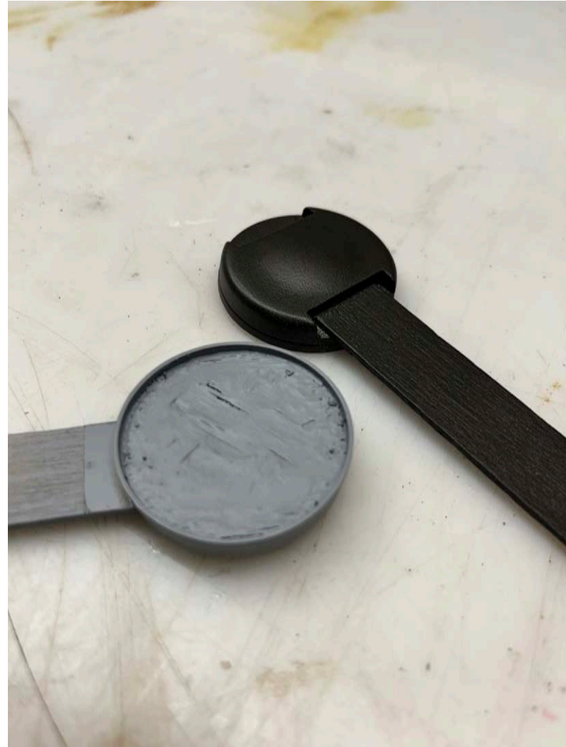
Monitor housing primed (Left), and painted (Right).
