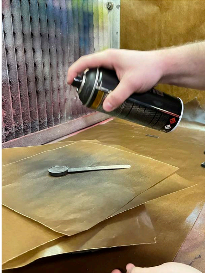
Wrist monitor housing was primed in preparation to be painted
